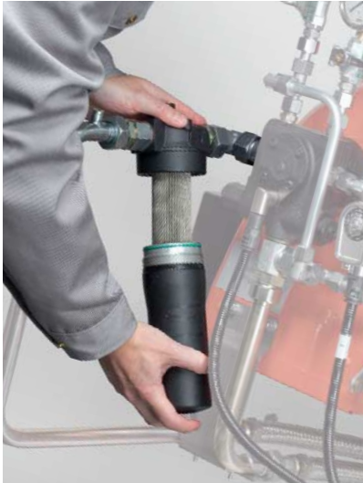
The integrated oil filter is easily accessible (standard on MS burners version with different MFO fuels in alternating operation)
