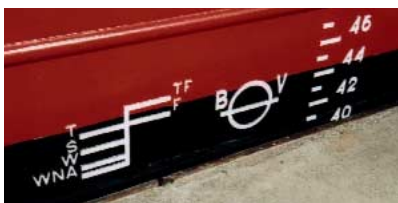
Classification identification by Plimsoll line
