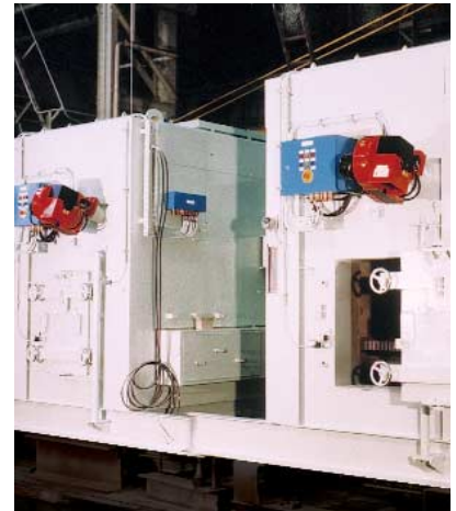
Waste incinerator on the luxury liner "MS Empress" with two L1 burners
